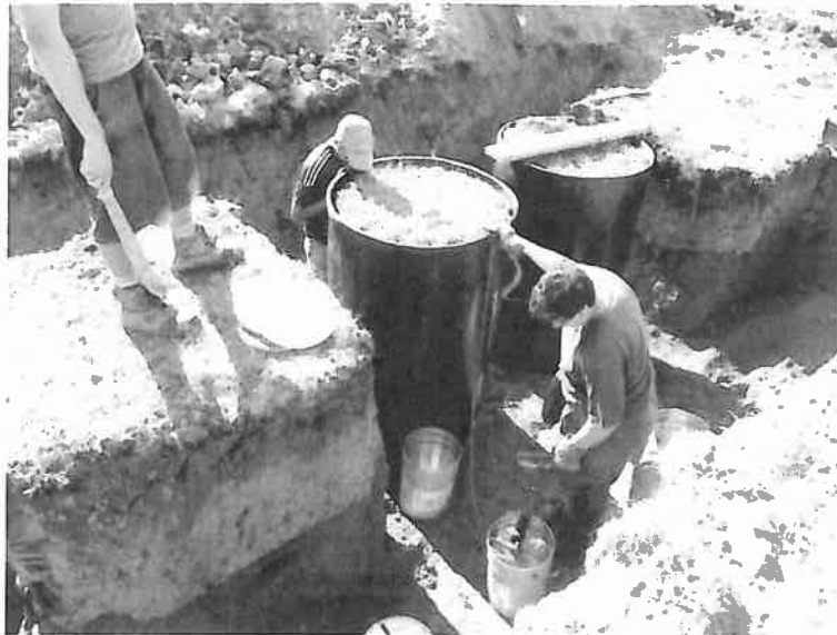
Figure 3. Sealing the edge of the soil with petroleum jelly to prevent edge flow.
