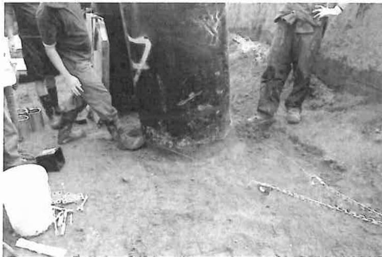
Figure 4. Using a wire to slice off the soil at the base of the lysimeter.
