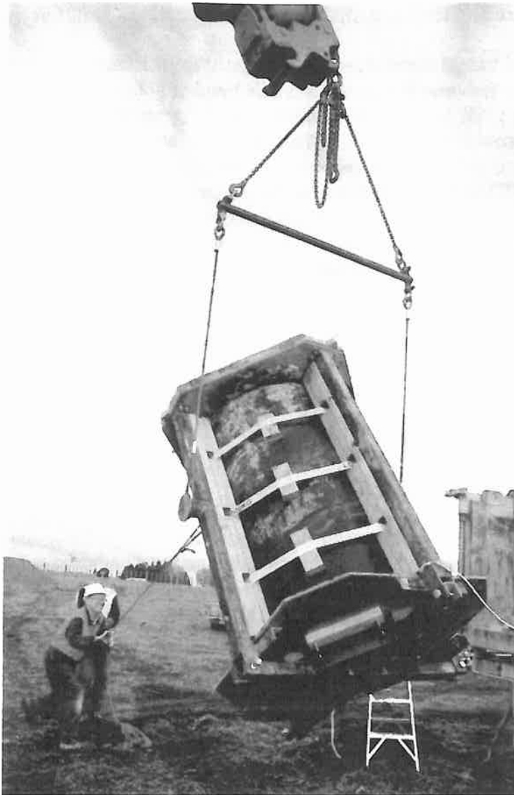
Figure 9. Rotating the lysimeter before attaching the fibreglass wicks.
