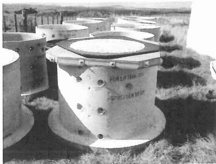
Figure 7. Lysimeter base system consisting of HDPE lysimeter base with wicks on the wooden base on concrete manhole riser.
