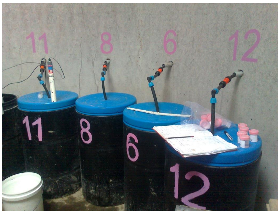
Figure 4 Leachate collection barrels in the underground facility.
