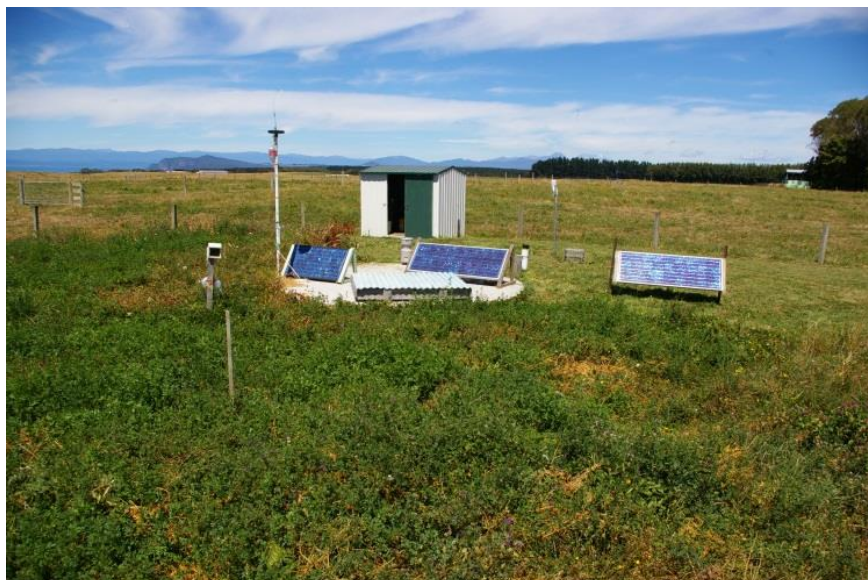
Figure 1 Lysimeter facility at Tihoi showing lucerne in the foreground and ryegrass/clover pasture in the background. Also visible are webcam, solar panels, cell phone aerial, rain gauges, roof of underground facility, and storage shed.
