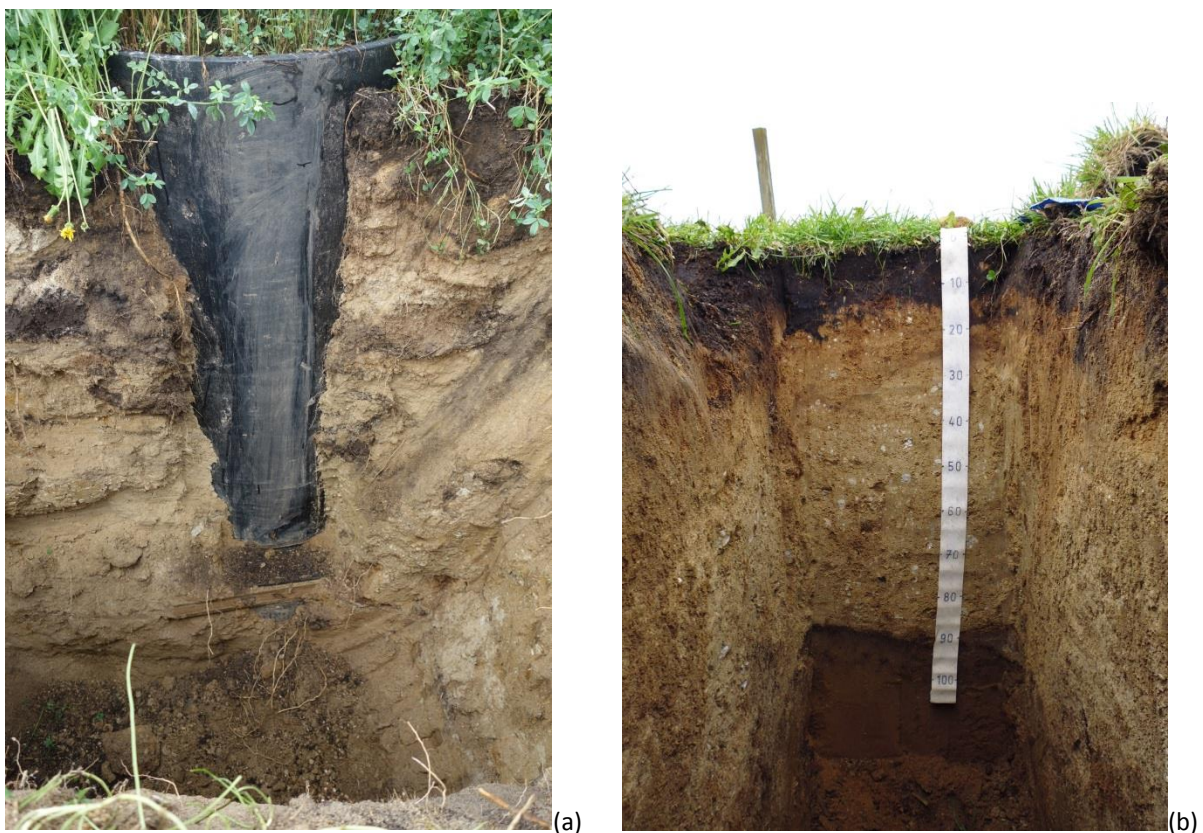
Figure 6 Rooting pattern of lucerne around a lysimeter (a) and ryegrass/clover pasture in a nearby paddock (b). Note the older volcanic silty tephra below 90 cm in the undisturbed soil.
