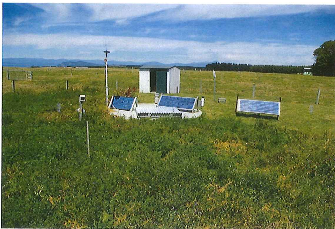
Figure 1 Lysimeter facility at Tihoi showing lucerne in the foreground and grass in the background. Also visible are webcam, solar panels, cell phone aerial, rain gauges, roof of underground facility and storage shed.
